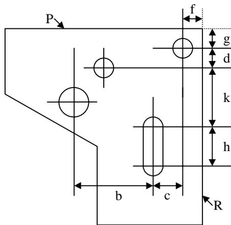
$f$  and  $g$  are measured using the height gauge from sides R and P respectively to the top of the plug gauge ( $d_3$ ).
