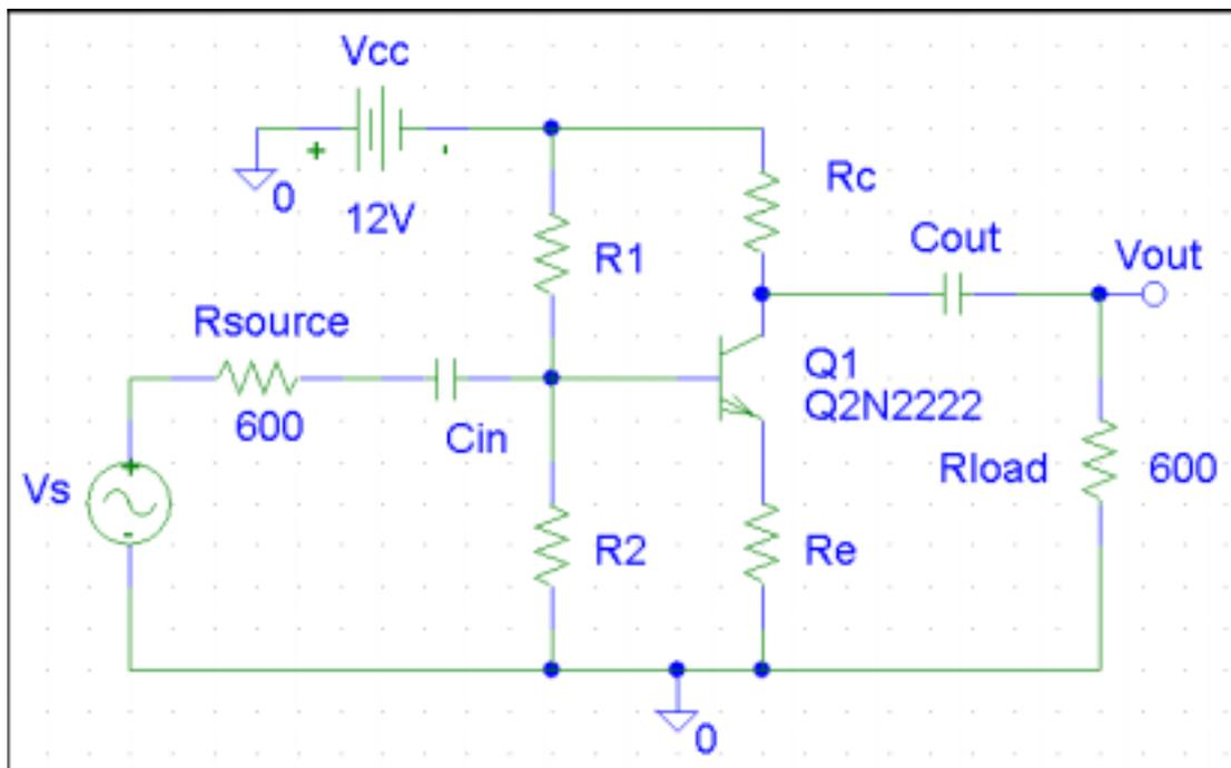
Since output impedance =  $\frac{1}{h_{oe}} \parallel R_c$  and  $\frac{1}{h_{oe}}$  is very large it can be assumed that output impedance =  $R_c$  and therefore  $R_c = 600\Omega$ . To maintain thermal stability  $V_{RE}$  should be 20-30% of  $V_{CC}$ .  $V_{CC} = 12V$  so a  $V_{RE}$  of 3V is chosen.
